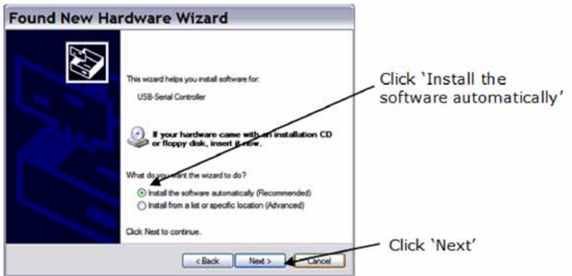
Figure 9. Installing drivers for cables
